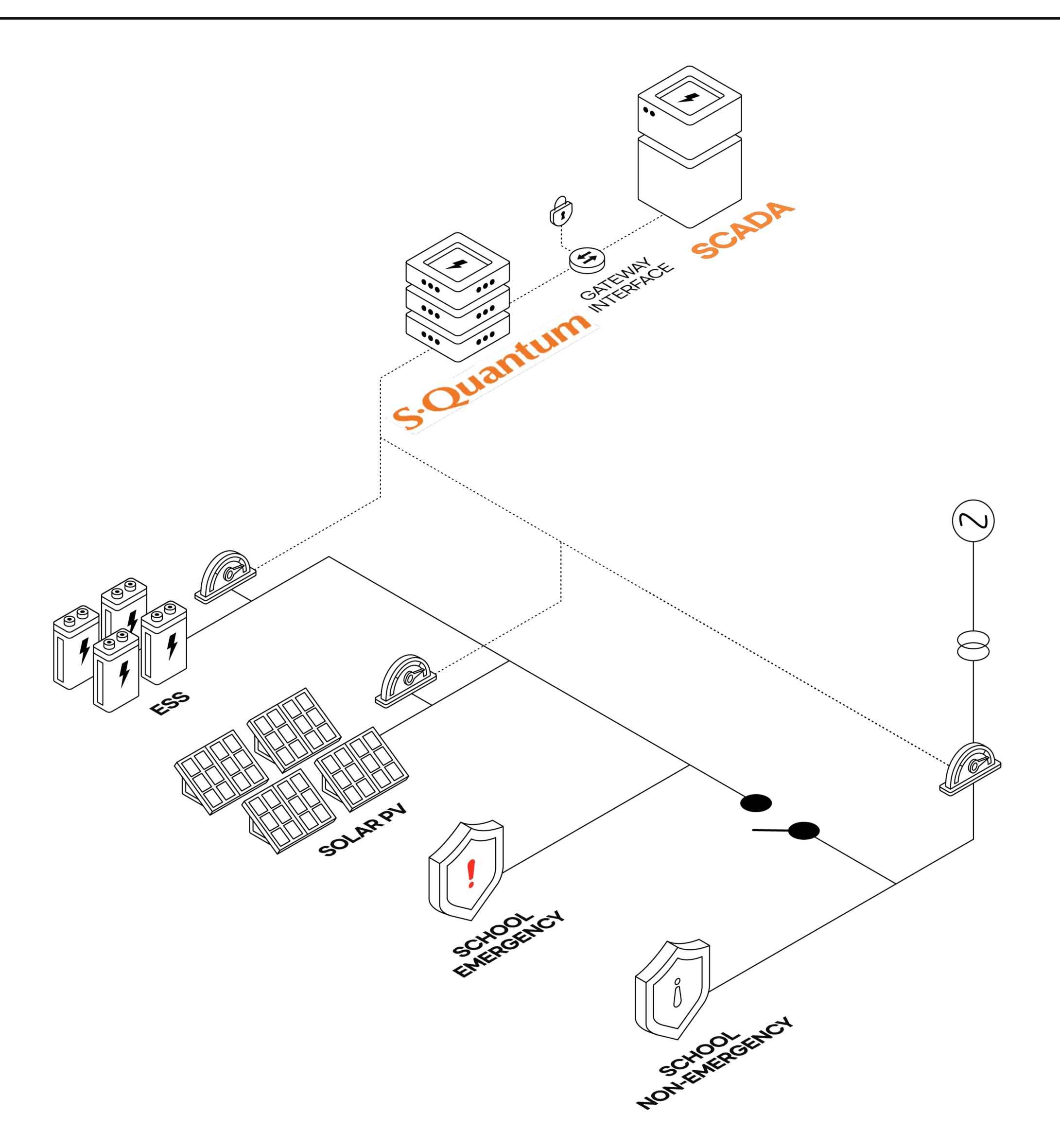
S-Quantum controls at multiple levels of distributed resources. Customers can manage at the Asset level, which is the ESS itself, or they may want to manage the entire site including the ESS, so there is no need for a separate ESS or Site controller as they can intervene at the required level with a single solution.
